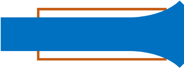
Fig. 9. Illustration of the beam (in blue) becoming wider during the propagation through an RF cavity (brown box) due to the RF deflection.
