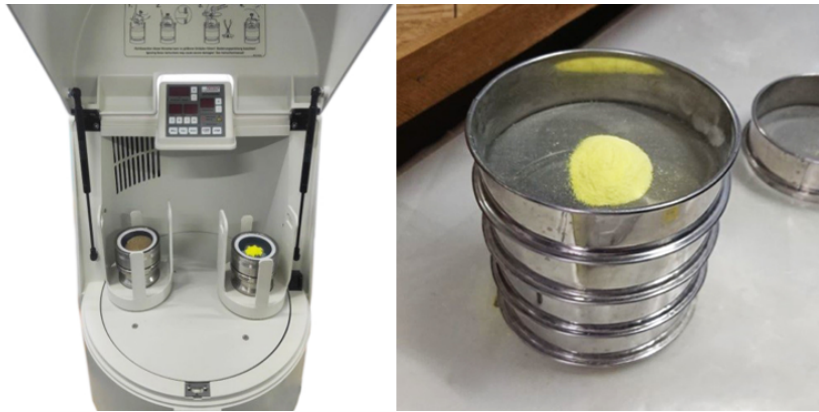
Figure 1: Left: Planetary mill Fritsch Pulverisette 5/2; Right: set of sieves for fractioning of the inorganic scintillation granules
