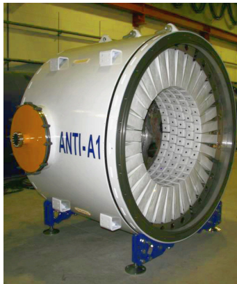
Figure 2.13: The first LAV station before placement in the vacuum vessel. Image reproduced from Ref. [67].
