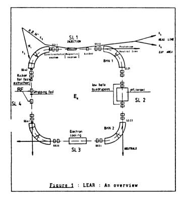
The antiprotons for LEAR, typically a bunch of up to  $3.0 \times 10^9$  particles, is unstacked from the AA and transfered to the PS, where the beam is decelerated from 3.5 GeV/c to 0.609 GeV/c, before being ejected towards LEAR. After about 3 minutes of stochastic cooling in LEAR at the injection momentum [609 MeV/c] the beam is either accelerated or decelerated to the required ejection momentum. At present, for ejection
