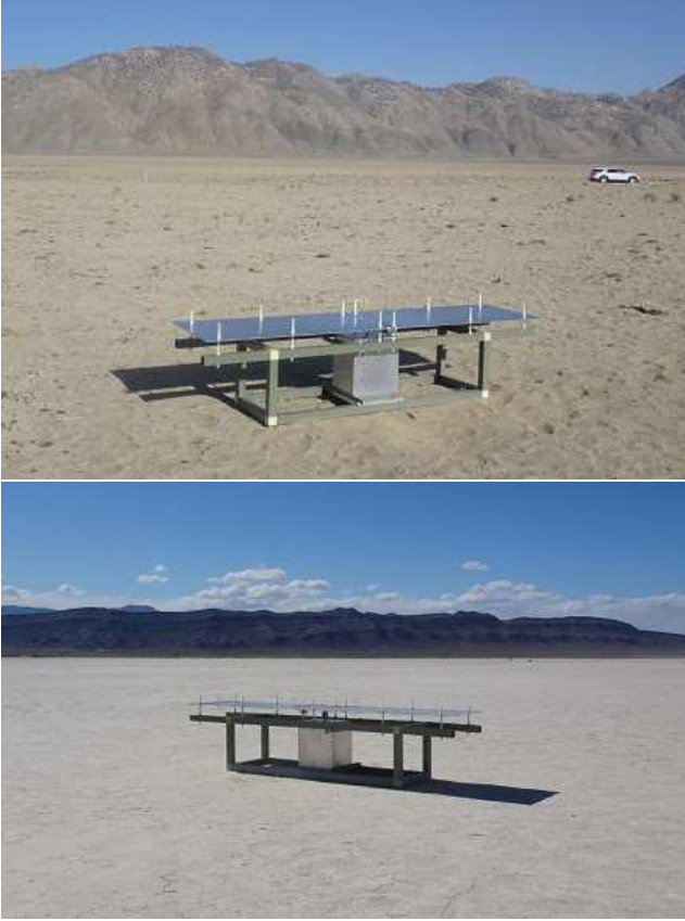
Figure 15. MIST instrument conducting test observations in Deep Springs, California (top), and in Death Valley, Nevada (bottom) in May 2022. MIST is a single-antenna total-power radiometer without a metal ground plane. The antenna is a blade dipole of 2.4 m tip-to-tip length and the measurements span the 25 – 125 MHz range. These test measurements are currently being analyzed to understand the diffuse synchrotron emission in the northern hemisphere as well as the effect of the ground on the sky measurements.
