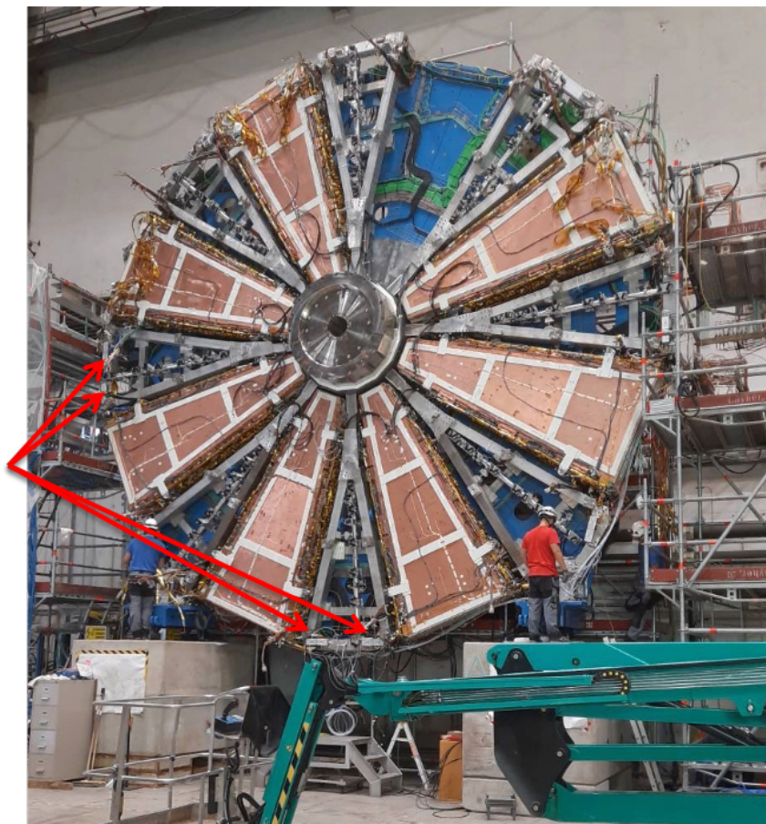
Figure 23: Placement of the LVD6R cooling bars on Wheel A, as shown by the red arrows.
