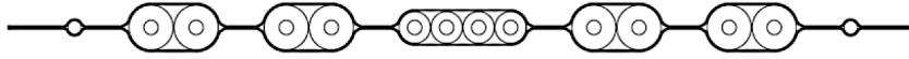
Figure 2: Cross-section of the MiniSAS twin-ax ribbon cable showing four pairs, four single-ended “side-band”conductors, the shield and two shielding drains. The cable dimensions are 15.6 \times 0.9 mm.
