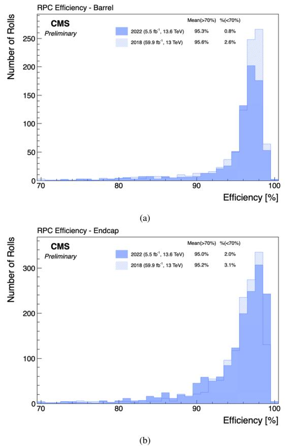
Figure 3: RPC overall efficiency distribution comparison for the barrel (a) and the endcap (b), obtained using 2018 and 2022 proton-proton collisions data.
