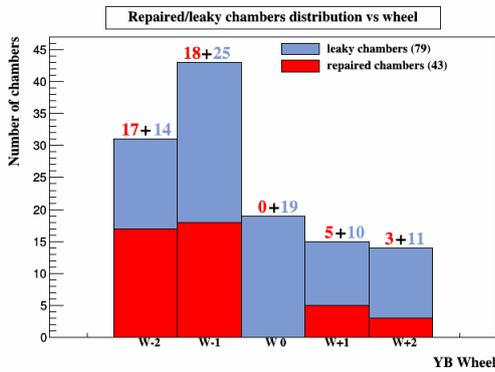
Figure 2: Distribution of leaking and recovered gas channels per wheel - representing the system in June 2022: 122 gas leaks out of which 14 non-recoverable leaks, 63 disconnected operational leaking chambers, 2 leaking chambers still connected and 43 leak repaired cases.
