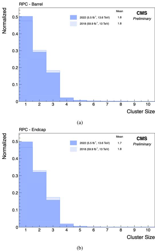
Figure 4: Cluster size distribution of RPC hits associated with muons in the barrel (a) and the endcap (b), based on data taken during 2018 and 2022 proton–proton collisions.
