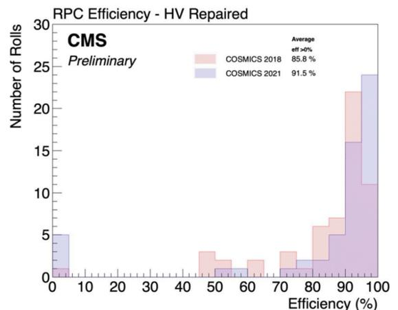
Figure 1: RPC Barrel efficiency comparison between cosmic runs taken in 2018 (Red) and 2021 (Blue).
