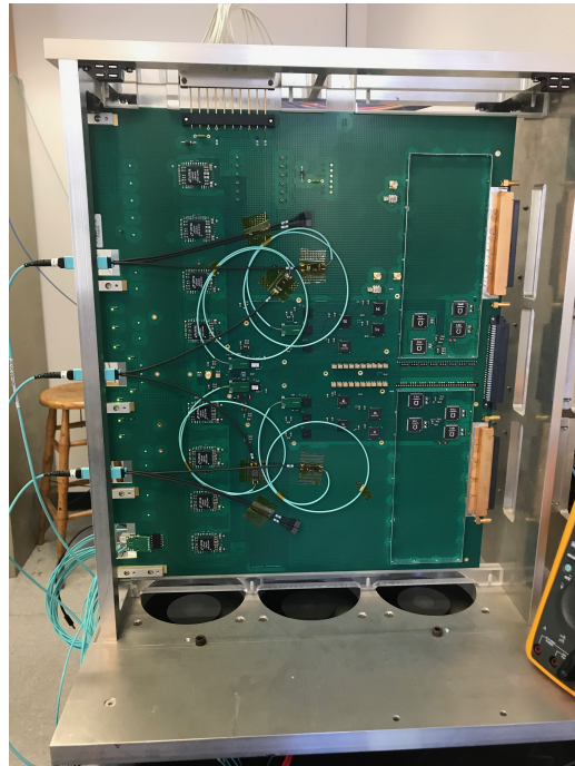
Figure 2: Photograph of the FEB2 Slice Test Board. This is a full-size pre-prototype test board for the FEB2 featuring a quarter of the channels (32 instead of 128) and with pre-prototype versions of the ASICs (8 Pre-Amp and Shaper ASICs: LAUROCv2, 8 ADC ASICs: COLUTAv3, 8 lpGBTv0). The ASICs are placed in the same density as on the full 128 channel board.
