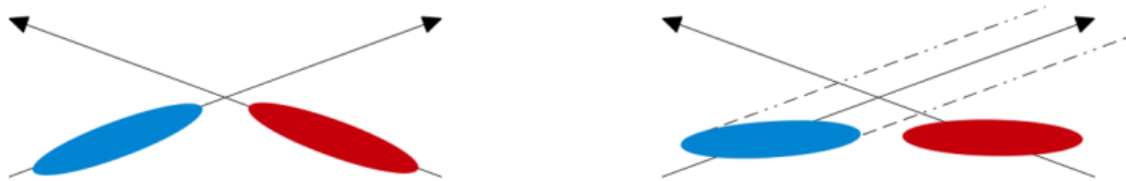
Figure 2. Bunches colliding with a crossing angle without crabbing (left) and with the crab crossing (right) [3].
