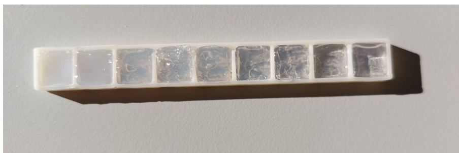
Figure 3. Samples of 3D printed plastic scintillator obtained with different opacity to visible light.
