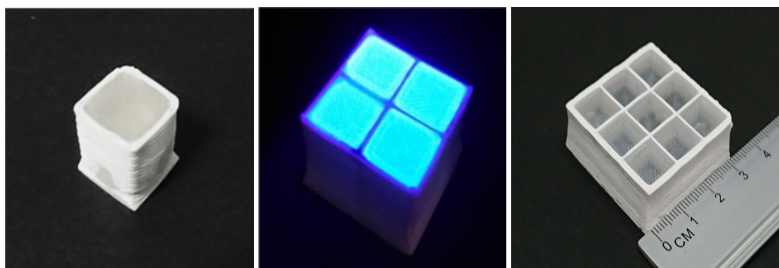
Figure 7. Left: polystyrene-based scintillator cube with optical reflector. Middle: 2 \times 2 cube matrix layer exposed to UV light. Right: 3 \times 3 cube matrix layer. The plastic scintillator cubes are optically separated by 1 mm thick reflector.
