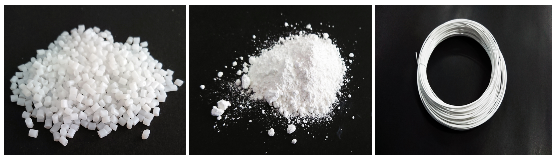
Figure 4. Reflective filament obtained by mixing polymer pellets (Left) with \text{TiO}_2 white reflective pigments (Middle) and then extruded to filament (Right).
