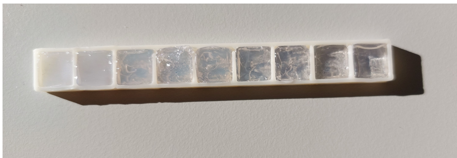
Figure 3: Samples of 3D printed plastic scintillator obtained with different opacity to visible light.
