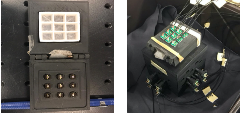
Figure 8: Left: 3D printed matrix layer setup, Right: setup used to selected vertical muons and evaluate the performance of 3D printed matrix layer. The second box is hosting glued-cube layers read out by WLS fibers and MPPCs.
