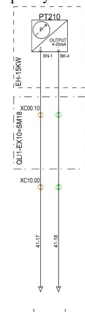
Figure 2: Block example : 4..20mA pressure sensor
