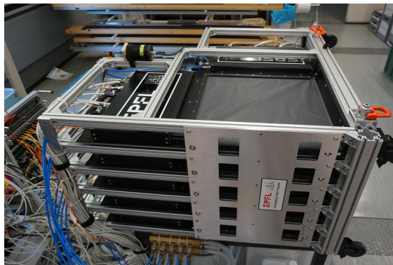
Figure 8. The SciFi tracker detector setup in the lab for cosmic ray test. The active area of a tracker module is 40 cm \times 40 cm and consists of 5 xy fibre planes.
