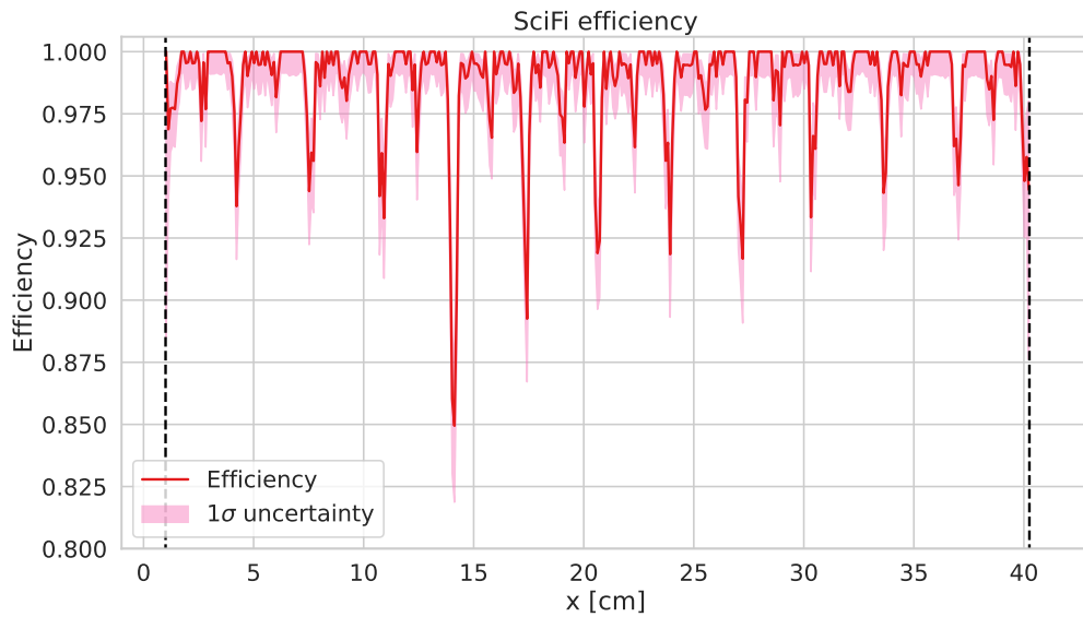
Figure 43. Efficiency of the x layer of the third SciFi module. The dips in efficiency are caused by the gaps between SiPM arrays. The black dashed lines indicate the edges of the layer.
