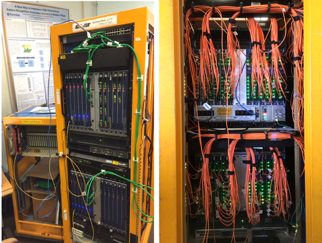
Figure 9. Demonstrator hardware rack. The Data Source boards are in the lower ATCA shelf and the PRBs are in the upper shelf. The rear view of the rack (right) shows 120 QSFP+ optical cables connecting the two shelves..
