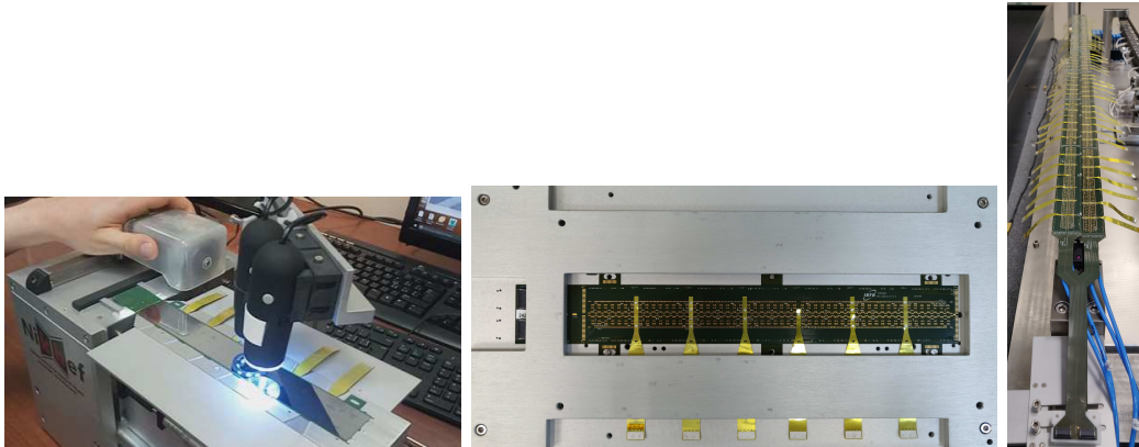
Figure 1. An OB HIC at the reception test. Center: the HIC is contained in a carrier plate which allows transport, storage, powering, testing, and vacuum gripper placement for handling. The left side of the HIC shows the so-called “tab” used to connect the sensors to the readout system. Once the HIC is qualified for alignment and gluing, the tab has to be cut as shown in the leftmost photo. Right: the two HS assembled in a stave: the sensors are glued directly on the carbon fiber strips. The blue pipes are the embedded water cooling lines (input and output). The HS are read-out by soldering an extension tab which is the interface with the outside world of the 98 ALPIDE chips. It can be clearly seen that the two HS come in different flavors (upper and lower) which have a partial longitudinal overlap requiring a definite sequence of installation.
