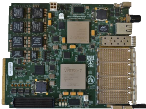
Fig. 5. Picture of the double AMC Tile PreProcessor Demonstrator [10].
