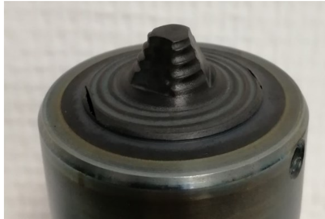
Figure 1. Friction stir welding tool (70% PcBN/30% W-Re), with a 8 mm long conical pin and 25 mm diameter convex shoulder.
