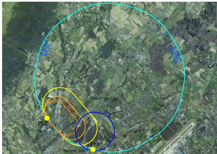
Fig. 14. Three racetrack alternatives proposed for the eh machine at LHC Point 2
