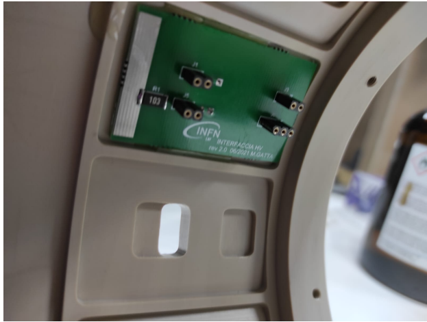
Figure 3.22: A HV distribution board glued on the flange.
