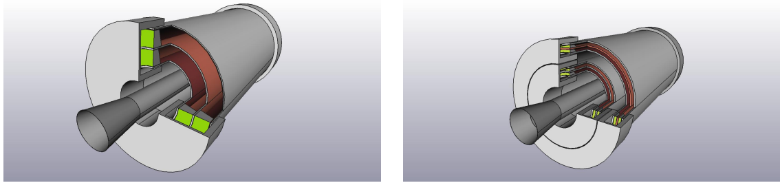
Figure 3.15: Inner Tracker ideas: double large gas gap (top) and pair of double thinner gas gap (bottom).
