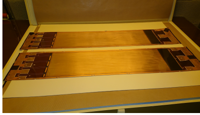
Figure 3.19: Flexible \mu -RWELL_PCB detector tiles manufactured at the CERN-PH-DT Workshop .
