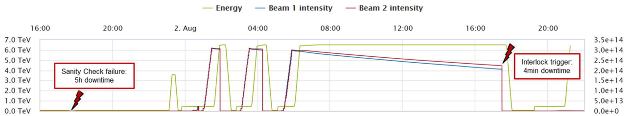
Figure 3: AFT extract of the 02.08.2017. Two distinct BLM failures with different availability and luminosity impact.
