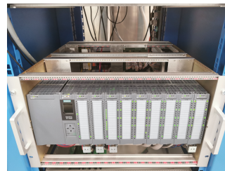
Figure 5: Left: PLC interlock unit. The back of the rack hosts signal conditioning cards and connectivity to patchpanels. Right: Excitation sources and interface PCBs for prototype connectivity
