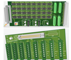
Figure 5: Left: PLC interlock unit. The back of the rack hosts signal conditioning cards and connectivity to patchpanels. Right: Excitation sources and interface PCBs for prototype connectivity
