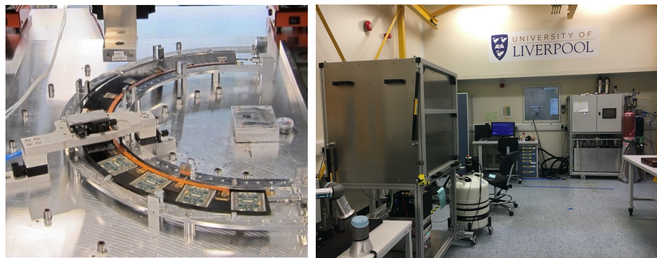
Fig. 6: (Left) Loading of RD53A pixel quad modules onto an end cap 'half ring' local support at RAL (UK). (Right) The outer endcap test stand with Lukasz CO2 cooling plant in Liverpool (UK).
