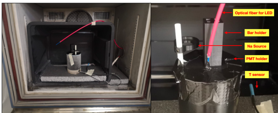
Figure 18. (left) A picture of the experimental bench used for the characterization of single crystal bars at cold temperatures. The bench is inserted in a thermostatic chamber able to provide stable temperatures down to -40^{\circ}\text{C} . (right) A detailed picture of the setup components.
