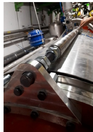
Figure 8: Additional tie-rod implementation in the LHC.
