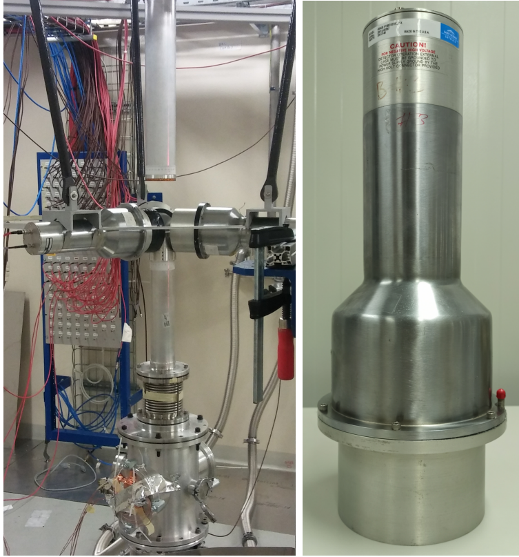
Figure 2.7: Left: The three BICRON detectors used to detect the (n,\gamma) cascades, in the lower part of the picture the chamber with the SiMon2 detector is shown. Right: BICRON C_6D_6 detector.
