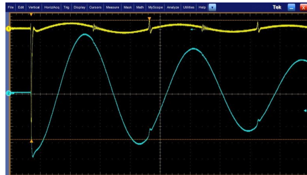
Figure 6: Measured voltages with generator at 1 kV: HV busbar (blue) 200 V/div, and DAG (yellow) 10 V/div. 20 \mu s/div.
