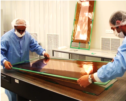
(a) Placing the first GEM foil in the stack.
