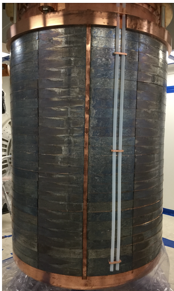
Extended Data Figure 2. Roman lead. Top left: the lead bricks recovery from the Sardinian sea. Bottom left: the ingot inscriptions were cut and preserved, while the ingot bodies were used for the CUORE internal lead shield. Right: Lateral view of the internal lead shield 21 .
