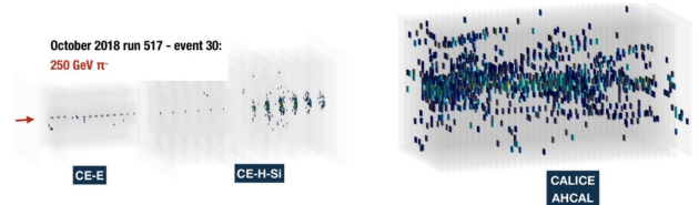
Figure 5: Display of a 250 GeV/c pion induced particle shower, recorded at a CERN test-beam in 2018. During this early campaign 6" silicon sensors for the CE-E and CE-H compartments were used.
