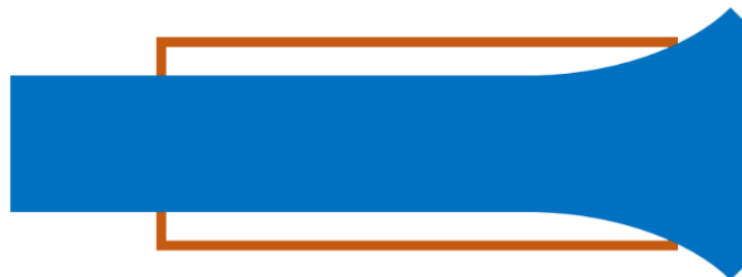
Figure 12: Illustration of the beam (in blue) becoming wider during the propagation through an RF cavity (brown box) due to the RF deflection.
