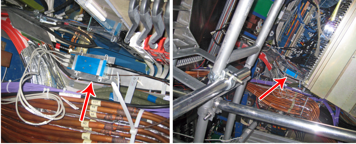
Figure 9. Example of the location of an MPX detector in ATLAS: MPX03 is fixed on a metal plate and surrounded by a batch of cables made of various materials which may have a significant influence on local radiation field at the position of the given MPX detector.
