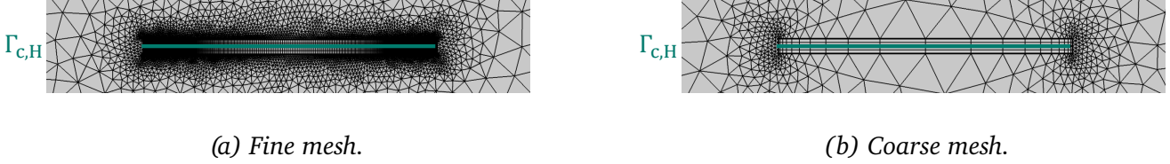
Figure 4.15. Mesh of the HTS tape, represented as a thin shell in the 2D setting. (a) Fine and (b) coarse mesh, for the low- and high-field and current scenarios.
