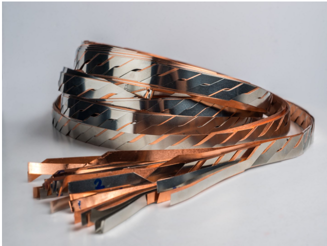
(a) Photograph of a coiled Roebel cable (by Henry Barnard). Figure taken from [2], © CERN.
