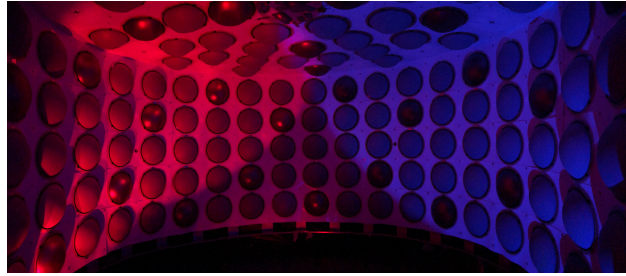
Figure 92. The interior of the CCM200 detector. Of the 200 PMTs, 80% are coated with wavelength shifter (TPB) to shift 128 nm scintillation light to the visible, leaving 20% uncoated (darker, more reflective PMTs in image), aiding discrimination of Cherenkov light. TPB foils cover the walls. The light-tight interior is surrounded by a veto region instrumented with PMTs. CCM is now running.
