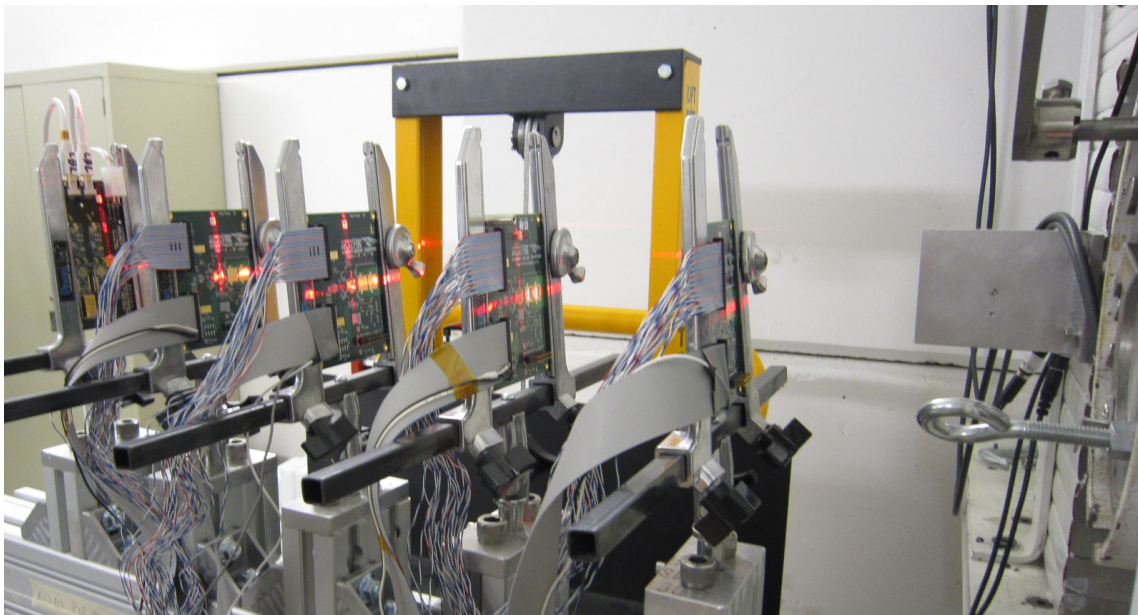
Figure 4. A picture of the setup used in the December 2020 proton beam test. The beampipe is visible on the far right, and the four PCBs to its immediate left correspond to SCBs with ABCStar ASICs mounted. Each SCB is connected to flat and twisted ribbon cables for slow and fast signals, respectively. The red laser focused on the ABCStar ASICs indicates the position of the beam.
