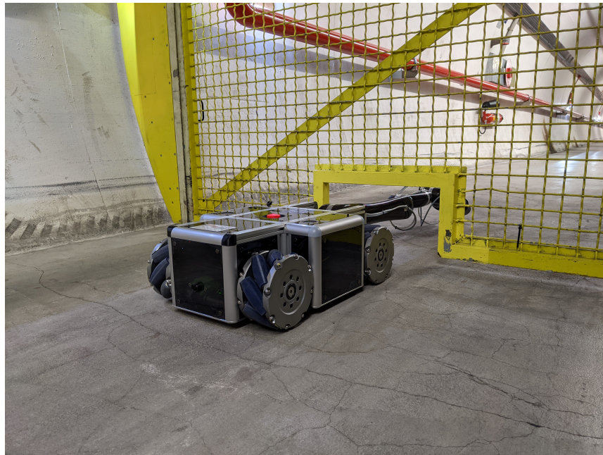
Figure 11. SPS robot crossing the door during the first test.
