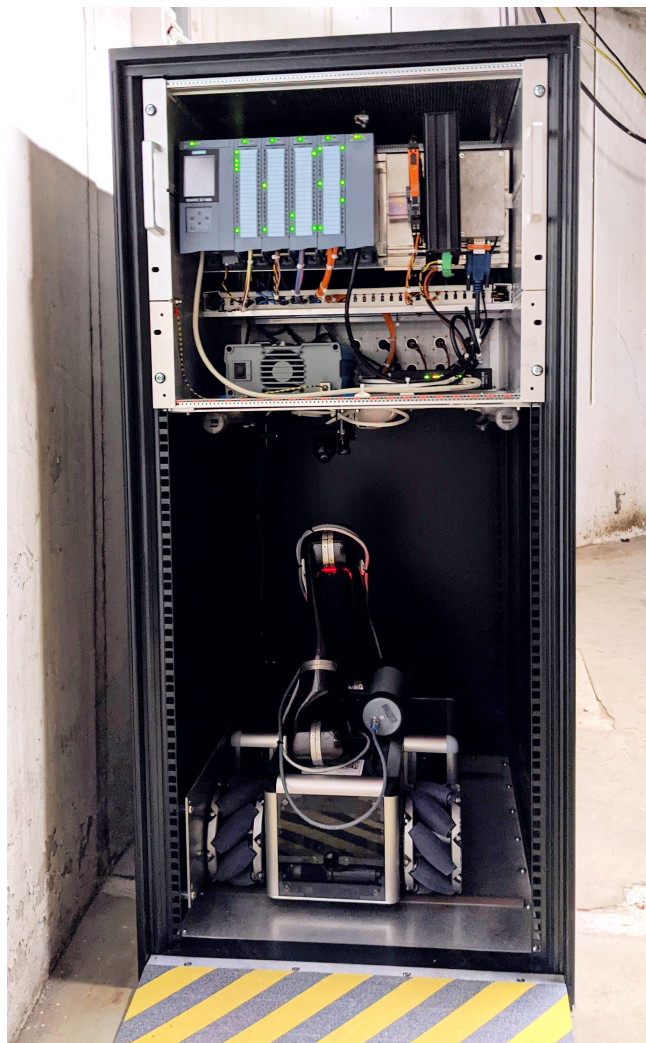
Figure 12. Robot in the charging station with the robotic arm folded over its top end plate.
