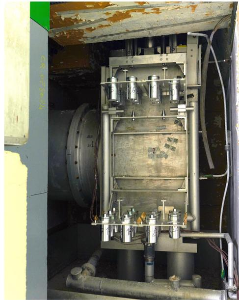
FIG. 5. Picture of the irradiation station, filled with samples, installed on the original target pool at n\_TOF NEAR. The top and the bottom shelves are visible. Four intermediate aluminum supports (two per shelf) with their handle for remote handling, accommodate up to six containers each. (CERN-PHOTO-202107-085-11) [39].
