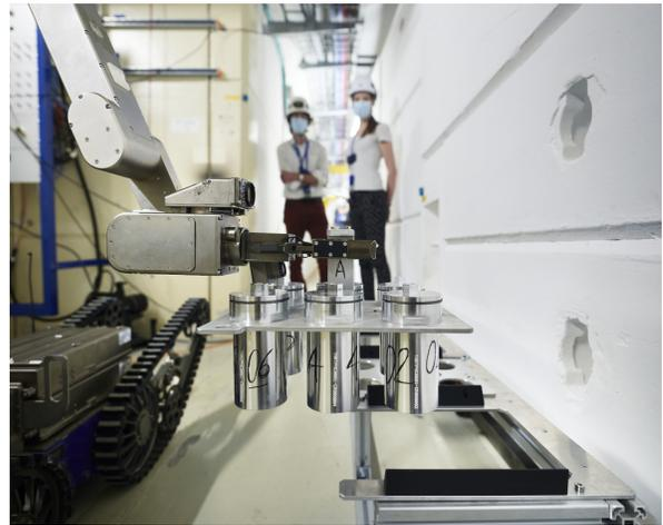
FIG. 10. Telexmax holding a support structure containing six samples of materials for installation (CERN-PHOTO-202107-085-1) [39].
