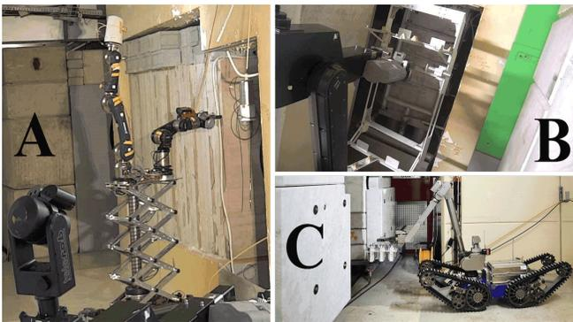
FIG. 9. Three of the main tasks carried out by robots: A) CERNBot2.0 with double arm configuration cutting cables; B) Teodor installing the shelf structure on the n\_TOF's spallation original target pool; C) Telexmax robot installing an intermediate support with 6 sample containers in the NEAR irradiation station (CERN-PHOTO-202107-085-7) [39].
