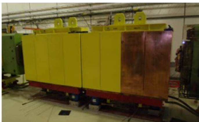
Figure 6. Picture of the 3.2 m long, water cooled, Fe-Cu based TAXes.
