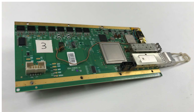
Fig. 2. Image of the OBBDT v1 prototype board for the time digitization of the CMS DT chamber signals.
