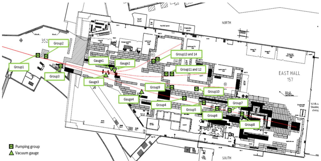
Fig. 4-17: Layout of the new vacuum system
