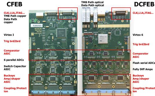
**Figure 5:** Cathode Front-End Board and Digital Cathode Front-End Board comparison
