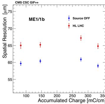
**Figure 7:** Spatial resolution of ME1/1 as a function of accumulated charge without additional background and with the equivalent average background occupancy at HL-LHC luminosity of  $5 \times 10^{34} \text{cm}^{-2} \text{s}^{-1}$ . Spatial resolution is stable.
