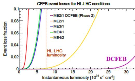
**Figure 4:** CFEB and DCFEB event loss for HL-LHC conditions. The dashed line is the anticipated luminosity at HL-LHC, below which CFEBs in ME234/1 will experience event loss. DCFEBs perform well-above this luminosity.
