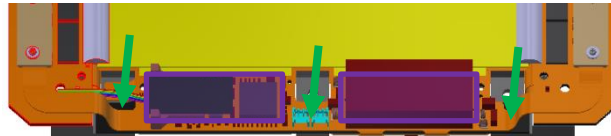
Figure 14. 2S-SEH in a module. Green arrows point to cooling locations. Purple boxes show the location of compensators.
