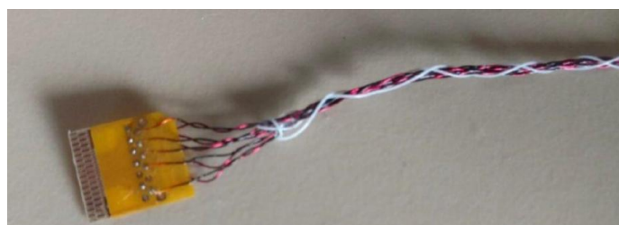
Figure 2. One end of a twisted pair electrical link (e-link).
