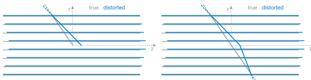
Figure 5: Diagram demonstrating distortions of the tracker geometry that may not affect the consistency of a reconstructed collision track with the measured hits (left), but introduce a kink when reconstructing the two halves of a cosmic ray muon track (right), leading to an inconsistency. This illustrates the telescope effect from Table 1.
