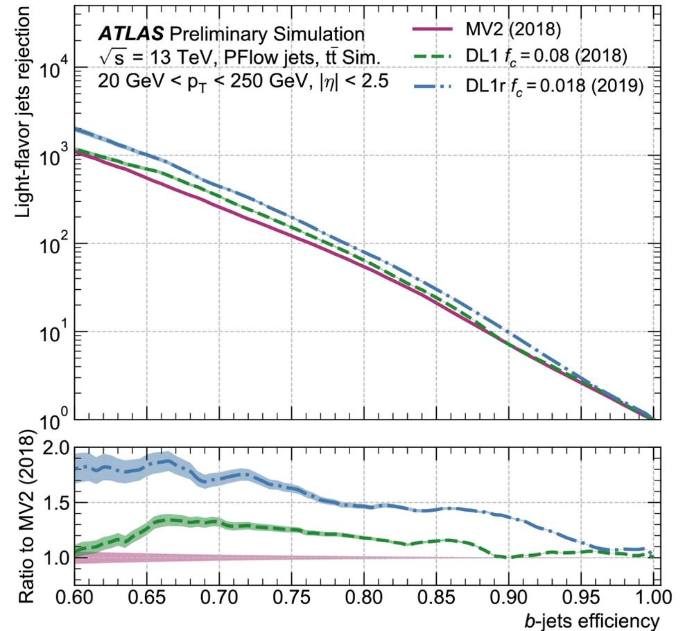
b-tagging: multivariate method for identifying jets coming from bottom quarks, combines information from track impact parameters, and secondary vertexing
