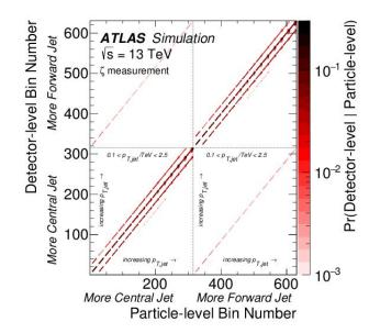
Unfolding by 2D iterative Bayes method (1 iter) sandwiched by explicit in/out migration corrs.
