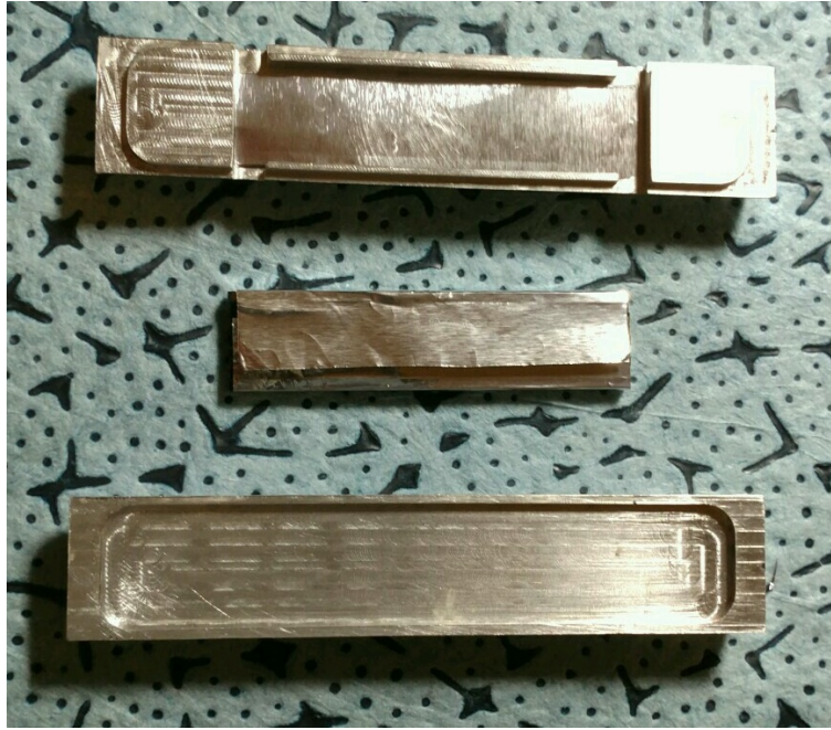
Figure 3. Photograph of the nine silicon crystal samples wrapped in an aluminum protection foil (in the centre) ready to be closed in the irradiation capsule (up and down).
