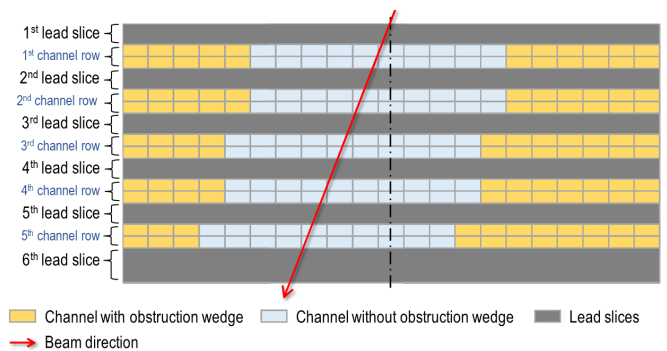
FIG. 11. Schematic view of the main core assembly (see also Fig. 5) showing, highlighted in yellow, the channels with wedge-shaped obstructions. The obstructions partially restrict the flow in the channels located farther from the beam axis, increasing the flow rate on the regions of lead surface directly impacted by the beam.
