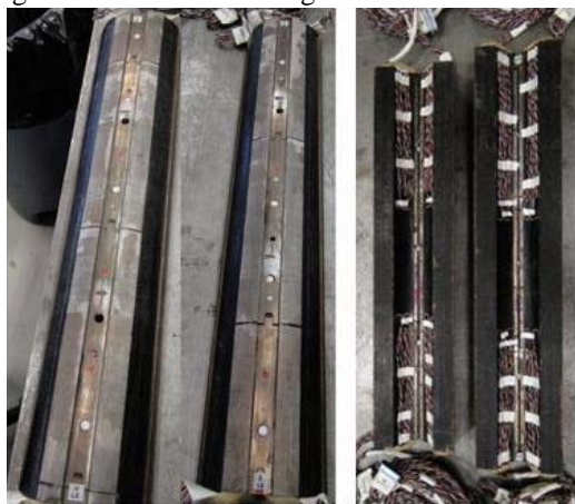
Fig. 2. Two instrumented central sections used for mechanical model assemblies shown from top and bottom.
