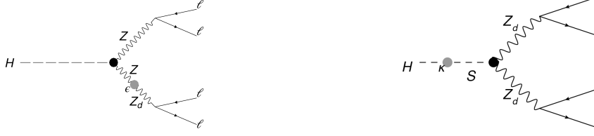
Figure 1: Exotic Higgs boson decays to four leptons induced by intermediate dark vector bosons via (left) the hypercharge portal through \epsilon and (right) the Higgs portal through k , where S is a dark Higgs boson [3].
