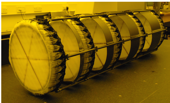
Figure 12. Photograph, with UV-filtered light, of one of the MICE trackers, showing the five stations. Each station has three doublet planes of scintillating fibres, each plane at 120^\circ to the next (the central fibres of each plane can be seen as darker lines traversing the station).
